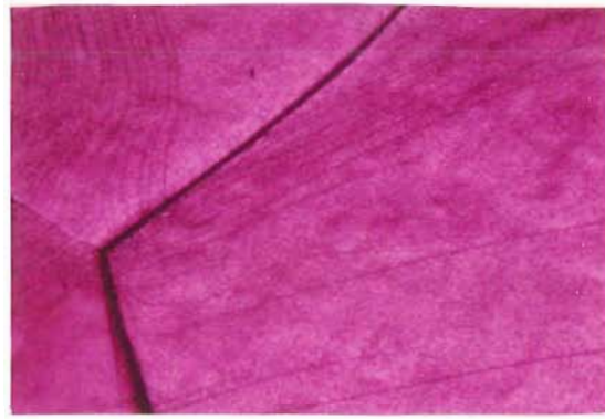
Figure 11. Suspected cracking in cavity #4SM
