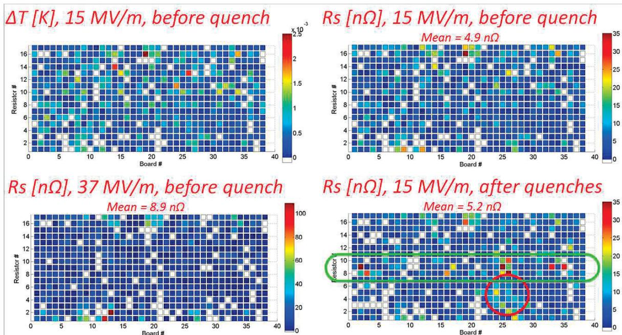
Figure 4: T-maps at low and high fields before and after quenches. The red circled area indicates the high field quench region and the green circled area indicates the mid-field quench region. Color scale in after-quench picture is forced to the same as before-quench, so some red spots may have higher  $R_s$  than indicated.
