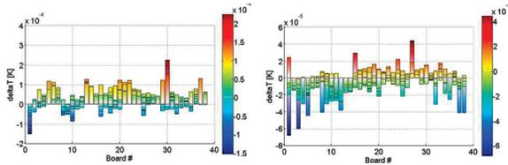
Figure 2: Approximate noise level for 1 measurement is  $2 \times 10^{-4}$  K (left), but by averaging 16 measurements, it drops to  $4 \times 10^{-5}$  K (right)
