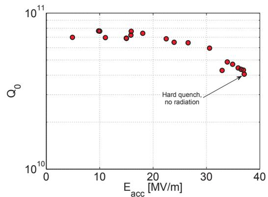
Figure 1: Cavity showing T-map setup (top) and its  $Q$  vs  $E$  curve at 1.6 K (bottom).
