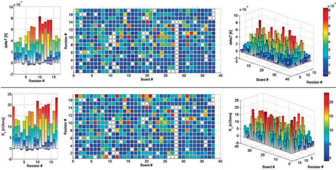
Figure 3: Top:  $\Delta T$  at 1.6 K, 10 MV/m,  $Q_0 = 6 \times 10^{10}$ , roughly 0.16 W total power dissipated! Average of 36 T-maps. Bottom:  $R_s$  calculated from  $\Delta T$  using dissipated power from RF measurements and surface magnetic field distribution from simulation. The average  $R_s$  is 5.4 n $\Omega$
