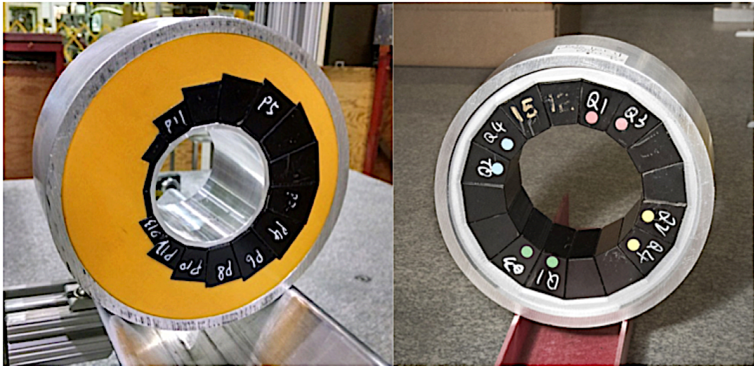
Figure 10: Defocusing (left) and focusing (right) Halbach prototype magnets for CBETA E_{\text{max}}=250 MeV.
