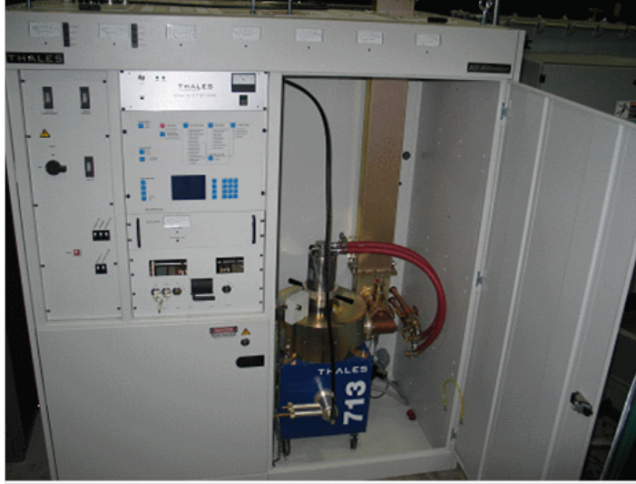
Figure 4.4.3: IOT inside the transmitter.
