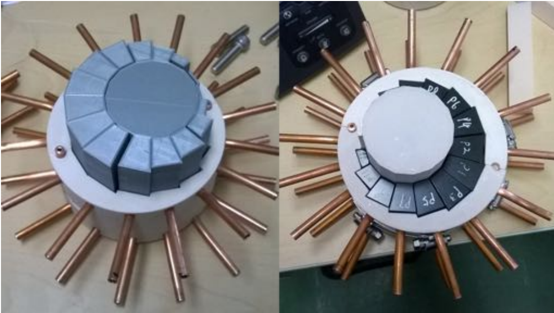
Figure 3.3.1: Previous assembly of the permanent magnet block. One by one they replaced the 3D printer plastic molds.
