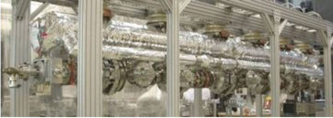
Figure 4.5.13: Beamline string hung from the GRP for the ERL injector .
