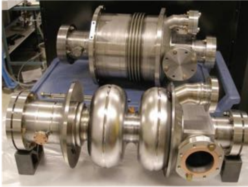
Figure 4.5.4: 2-cell cavity before and after welding the helium vessel
