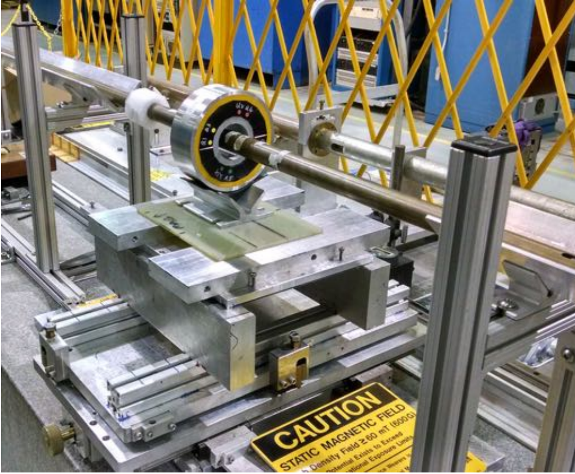
Figure 1.4.1: The Halbach FFAG magnet QF on a rotating coil test bench.
