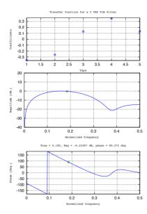
Figure 2: FIR filter Bode Plot. The frequency response has maximum magnitude 0 dB and phase 90 deg around  $\left[Q_{y}\right]=0.185$
