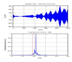
Figure 9: Vertical displacement vs. turns and fractional tune of a slice in the Tail of the bunch. The kicker signal saturates at  $2.874 \cdot 10^{-5}$  eV.sec/m. The instability grows larger and faster compared to the head. The tune is shifted to  $[Q_u] = 0.2152$ .
