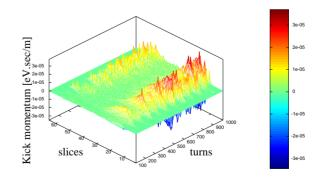
Figure 4: Momentum slices vs. turns, applied to the bunch by the kicker. The first 100 turns are cut off to avoid displaying the initial offset. Slices close to 0 represent the tail of the bunch, while slices close to 64 represent the head.
