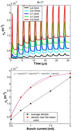
FIG. 6. Bunch current effect on electron build-up (top) and peak electron density (bottom) in a quadrupole magnet with a field gradient of 1.0 T/m
