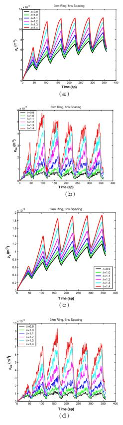
FIG. 7. Electron build-up in the ILC quadrupole magnet without ante-chamber protection. (a) 6ns spacing, average density; (b) 6ns spacing, electron density near the beam; (c) 3ns spacing, average density; (d) 3ns spacing, electron density near the beam
