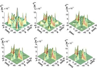
FIG. 3. Evolution of electron cloud during the train gap, frames separated by  $\Delta t$ =70 ns. Parameters used for simulation: Bunch length 17.24 mm, bunch current 1.0 mA, bunch spacing 14 ns, field gradient 0.517 T/m, peak SEY 2.0, energy at peak SEY 310 eV, photon flux 0.21 photons/m/particle, reflectivity 20%.
