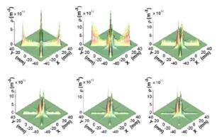
FIG. 5. Evolution of electron cloud during the train gap with a field gradient of 9.2 T/m. Other Parameters are the
