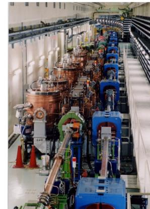
Extending of RF system for high beam current
