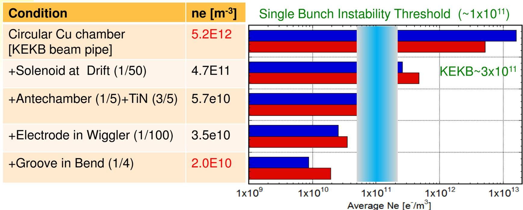
Low density in the simulation  $\leftarrow n_e=0$  by solenoid. Careful solenoid winding is important.
