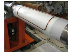
Superconducting magnet to shrink colliding beam at IP
