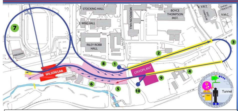
Key: 1=Photo-cathode Injector, 2=First-stage acceleration, 3=Turn-around arc, 4=Second-stage acceleration, 5=Accelerator test beamline, 6=South x-ray beamlines, 7=CESR turn-around arc, 8=North x-ray beamlines, 9=Cryoplant, 10=Electron beam stop
