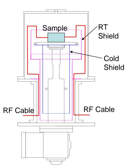
Room Temperature shield and cold shield are installed for RF cables not to see GM refrigerator directly and reduce heat radiation
