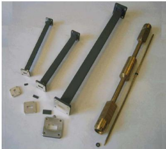
Figure 1: Transmission lines for 4 frequency ranges.
