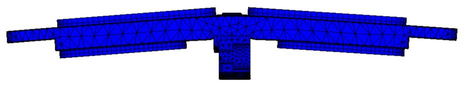
• large concentration of stress at edge of tile, near pivot point
