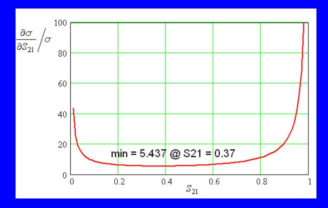
For accurate measurement of conductivity, the absorption in the waveguide should not be very small or too big, this can be adjusted by the length of the absorber.
