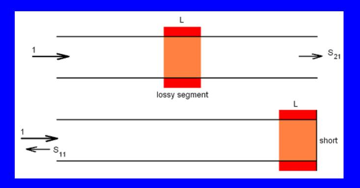
Formulas for dependence of conductivity on the S21 or S11, length and cross-section of a lossy waveguide, and frequency are derived in: http://www.lns.cornell.edu/public/ERL/2010/ERL10-1/ERL10-1.pdf
