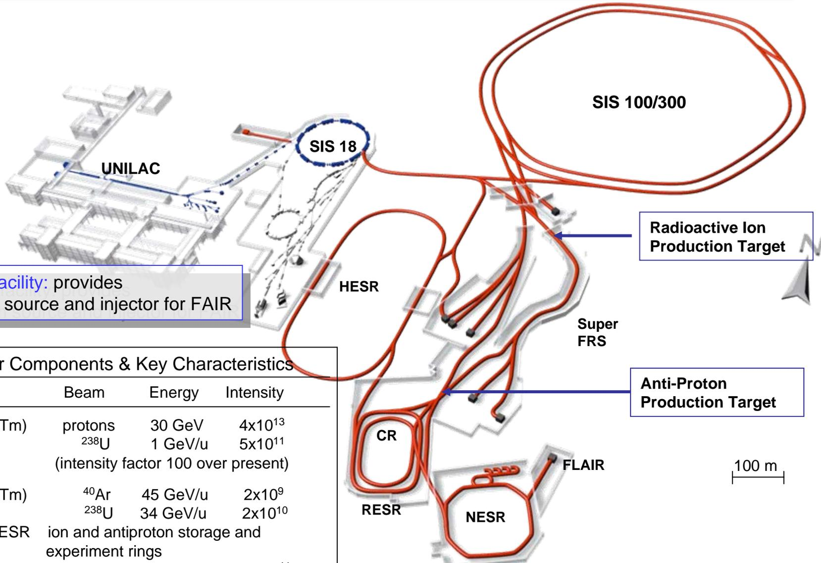
Existing facility: provides ion-beam source and injector for FAIR
