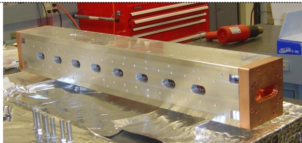
Figure 2. Undulator body on assembly bench in clean room in 12 GeV Annex.
