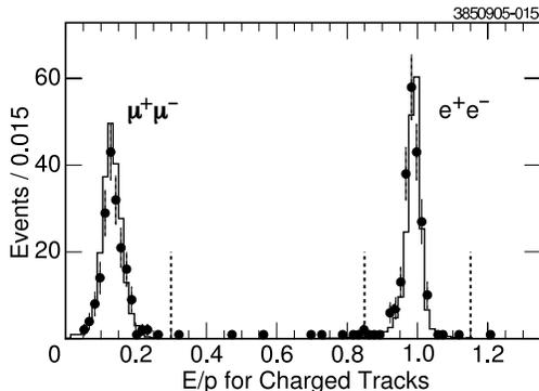
FIG. 1:  $E/p$  distribution of the charged tracks in data (points) and in the signal MC for  $e^+e^-$  and  $\mu^+\mu^-$  channels (histograms). Vertical dashed lines indicate the cut regions for electron and muon identification.
