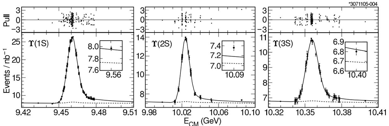
FIG. 4: The hadronic yield versus center-of-mass energy in the vicinity of the three  $\Upsilon$  resonances. Points represent the data, corrected for fitted beam energy shifts between scans, the solid line is the fit, the dashed line is the sum of all backgrounds, and the insets show high-energy measurements. The pull of each point is shown above.
