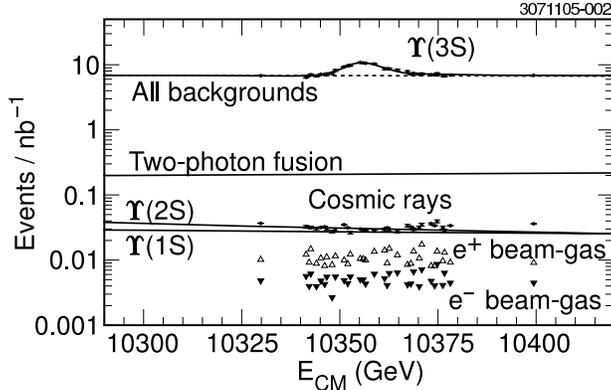
FIG. 2: The event yield as a function of center-of-mass energy in the region of the  $\Upsilon(3S)$ . The top points are data, with the fit superimposed, and the dashed curve represents the sum of all backgrounds. The lower points and lines show the individual non- $1/s$  background contributions.
