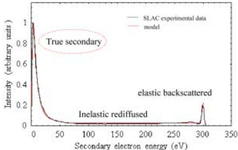
*Measured SEY, high-purity Al, degreased, NaOH etched and rinsed. (R. Kirby, SLAC).*
