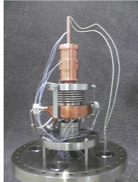
Fig.3: Photocathode cooling test-bench with temperature sensors and electrical heater on the top
