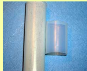
Tube before and after ethanol rinsing
