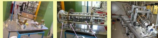
Alignment frame for sliding connector disc
