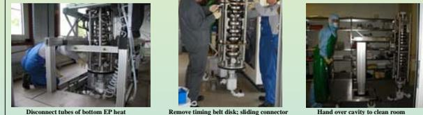
Disconnect tubes of bottom EP head
