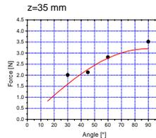
The measurements confirm the "sin" dependence of force and spot size from the angle. This is important once the cleaning effect on the curved cavity surfaces will be studied.
