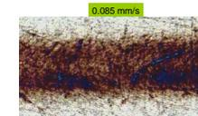
Effect of a moving jet ( $p=100$  bar,  $\sigma=0.345$  mm) impinging on a Nb sample with a speed corresponding to 10 s static jet. The presence of only small area of blue color agrees with the "10 s" static case.
