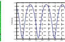
The oxide formation has been studied using monochromatic light and the theory of optical properties of thin film. The two pictures are the same as the top picture but illuminated by laser light at the reported wavelengths. This analysis method might help in determined the thickness of the oxide layer. In particular, at 543 nm a plot of the reflectivity vs oxide thickness is shown. The minima in reflectivity correspond to the dark rings in the picture.
