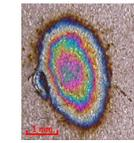
The effect of a prolonged exposition of the Nb sample to the HPR jet produces the formation of concentric ring of different colors, like interference fringes. We assume that the water jet effect is the growth of an oxide layer over the Nb surface.
