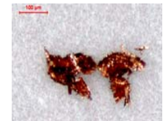
Copper particle detected on a filter disc Origin: Cu seal or CuNiSi nut
