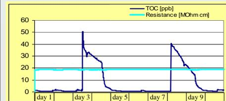
TOC data for maintenance on polisher ion exchanger
