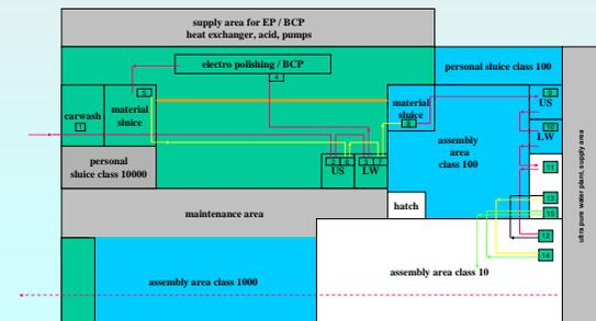
Proposal for a cleanroom lay out with minimum cross contamination by cavity work flow
