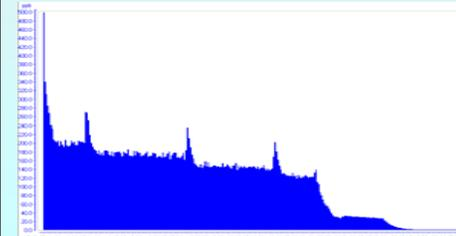
TOC data for qualifying a new supplier for ion exchanger TOC recovery time 6 days/ Resistance recovery 1h
