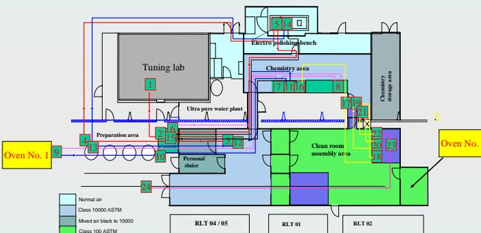
Workflow inside DESY cleanroom for cavity preparation => ELECTRO-POLISHING
