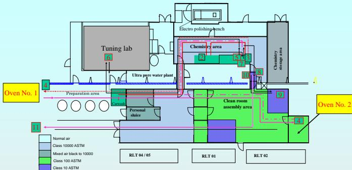
Workflow inside DESY cleanroom for cavity preparation => ANNEALING and TITANIUM POST PURIFICATION
