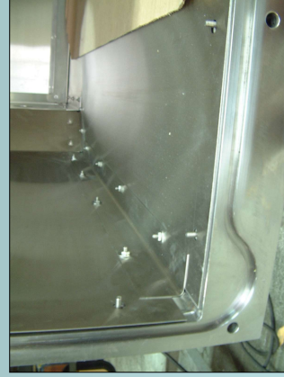
Magnetic shielding is provided by a single 0.040" thick layer of AD-MU-80 by Ad-Vance Magnetics, Inc. To simplify fabrication and installation, pre-punched shield sections are laid over threaded studs welded to the vacuum box interior. The overlapping sheet edges are secured with stainless steel batten strips to ensure intimate contact. Shielding on the lid compresses a spring-loaded shield angle attached at the box flange for good box-to-lid shield contact. The design goal of <20 mG residual field was exceeded, with measured fields not exceeding 16 mG in the spaces occupied by cavities. Shielding levels will further improve once large holes at the coupling ports are patched.
