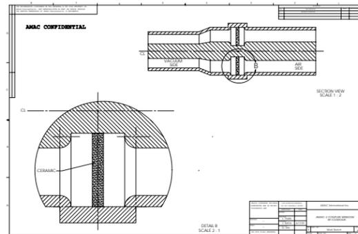
Figure 1 AMAC-2 coupler window geometry
