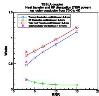
Figure 3 Cold Window Assembly: Conductive Thermal losses calculation results
