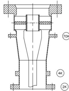
Figure 4 Cold window subassembly for AMAC TESLA coupler
