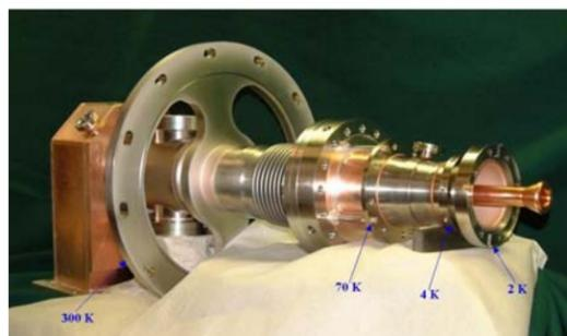
Figure 2 General assembly of TESLA coupler developed by AMAC and fabricated by CPI
