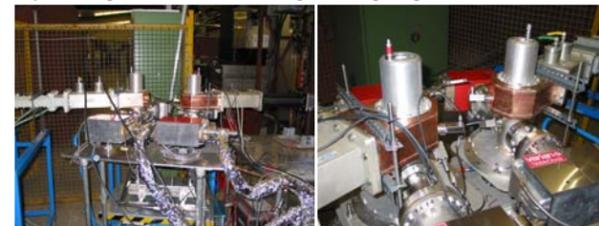
Figure 5: Couplers on the test stand.
