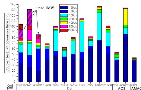
Figure 7 Couplers conditioning time: TTF3 and AMAC
