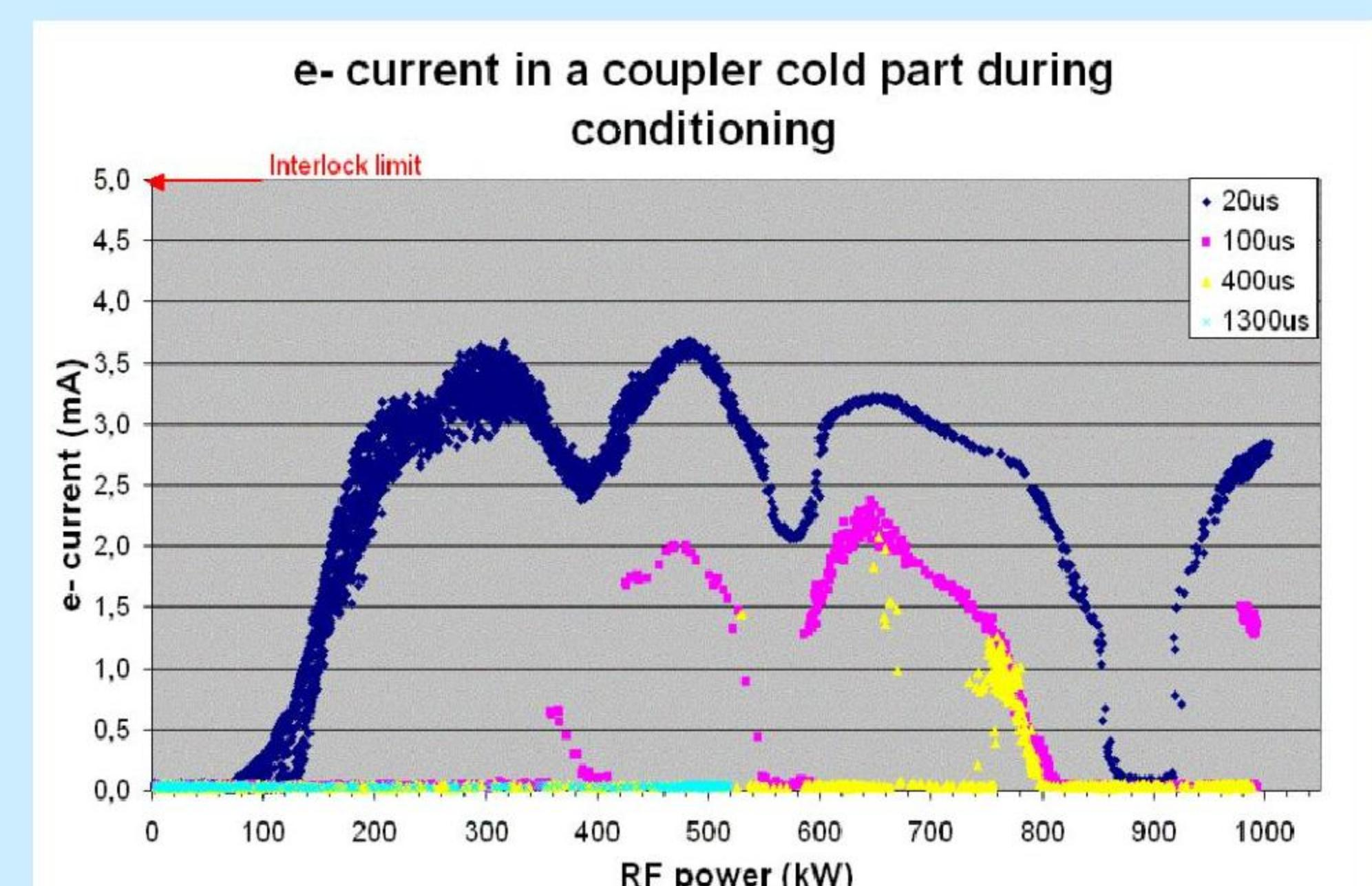
Conditioning acts on coupler surfaces causing a reduction of the SEE. This permits a progressive decrease of the e- currents during the coupler process.
