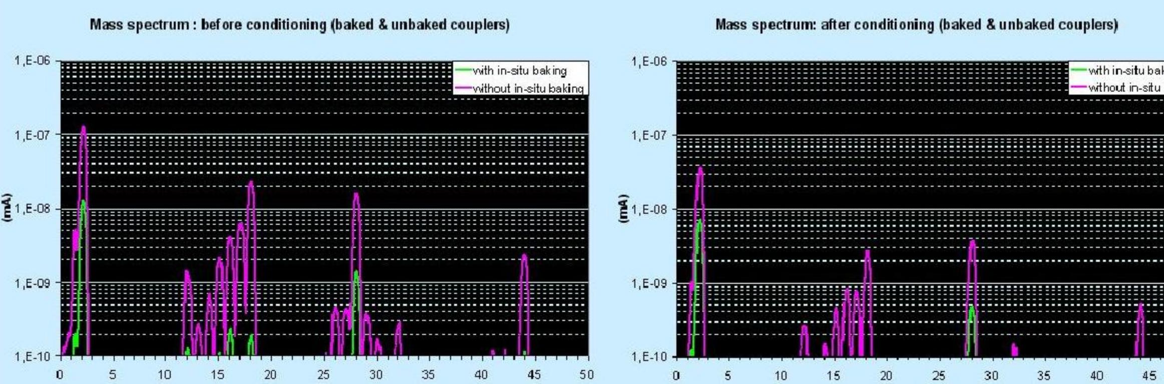
Mass spectrometry on coupler cold parts shows the effect of in-situ baking on coupler surfaces.
