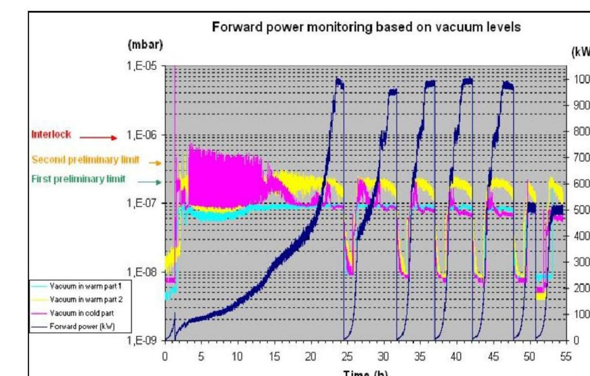
The most time consuming step during conditioning is the first one. Some powerful discharges can be seen especially at the first vacuum burst. This can activate a protection interlock which stops the RF power.
