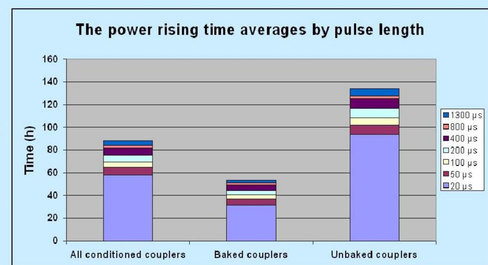
Averages done on 7 coupler pairs shows that one can save more than a half of the conditioning time by baking.
