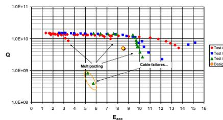
Three tests have been performed at JLAB on the cavity
