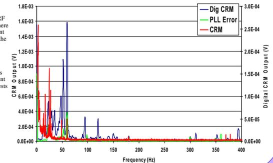
The digital system was used to measure an operating CEBAF SRF cavity. The results are compared here to an existing analog measurement system, and to a measurement of the PLL error signal. Since the measurements were not taken simultaneously, stochastic components differ between the measurements, but spectral peaks coincide at several known invariant lines (e.g. 27, 30, 59.5). Further tests of the improved instrument are planned.
