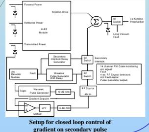
Setup for closed loop control of gradient on secondary pulse
