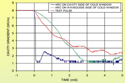
**TYPICAL DECAY TIMES FOR TWO TYPES OF ARC AND A TEST PULSE**
