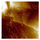
Initially the effects of BCP 1:1:2 etch depth on niobium roughness and step height between grains was studied. Roughness increases significantly between 50 and 100 um. We decided to use the standard 100um etch for the study.
