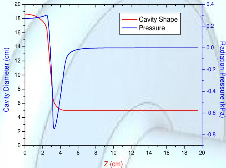
**Lorentz Pressure Deformation for 5 mm wall thickness**
