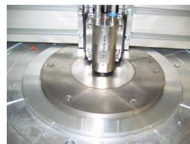
Scanning disks is part of the QC process during SRF cavities production:
