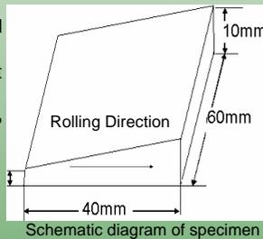
After rolling, the specimen was sliced along the rolling direction to make 8 equal size strips
