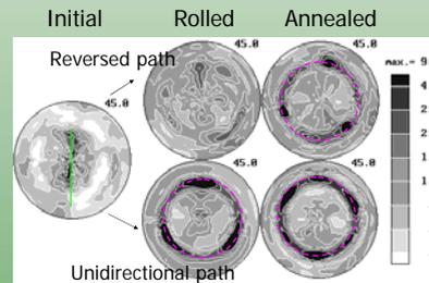
In the **center**, After rolling, the  $\alpha$  fiber decreased,  $\gamma$  fiber increased. After annealing, the  $\gamma$  fiber becomes very strong
