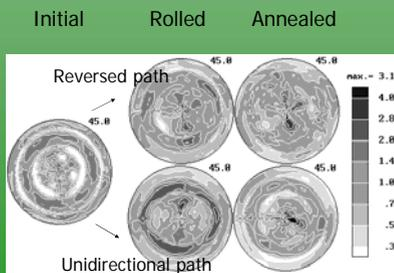
On the **surface**, After rolling,  $\alpha$  fiber unchanged, slight  $\gamma$  fiber increase. After annealing, the  $\gamma$  fiber weakened
