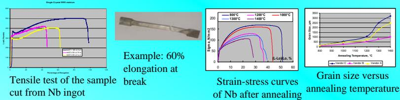
Grain grow in the polycrystalline Nb sheets guides by the reduction of the elongation at break. Large grain samples from Nb ingot demonstrate a very high elongation at break
