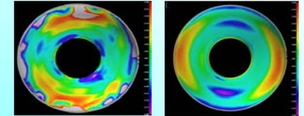
Deep drawing method proven as best for Nb sheets seems not to be appropriate for large grain Nb discs
