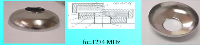
Half cell of TESLA shape deep drawn by one stiff and another flexible tool (polyurethane) The half cell is lick tight. The steps on grain boundaries are pronounced. Earing is pronounced (anisotropy of properties)
