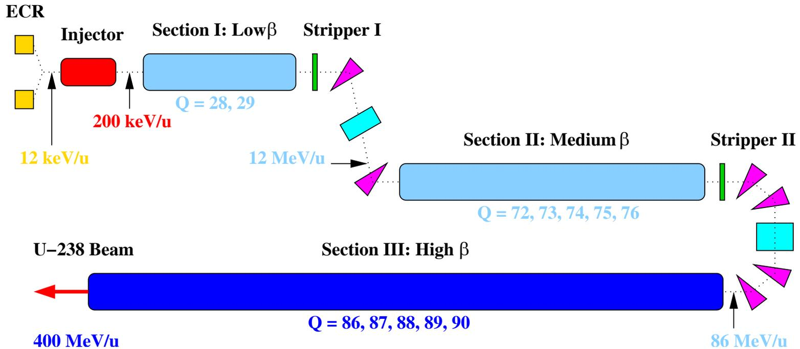
**Baseline:** About 1200 beam line elements: ~ 400 rf resonators, 90 solenoids, 100 quads, 16 bending magnets, ...
