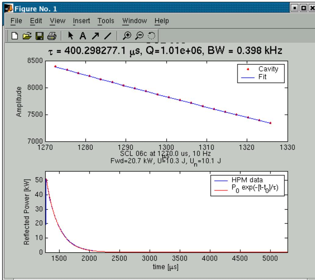
The field at the end of the pulse is determined via a measurement of the stored energy, calculated from integrating the emitted power
