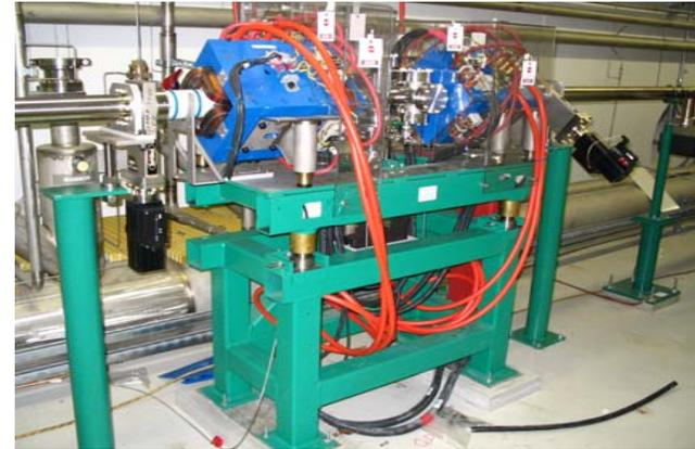
Warm section stand with beam pipe, magnets and diagnostics
