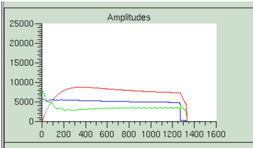
Reflected and Transmitted amplitudes change drastically after a quench: The coupling changes from about 1000 ( $Q_L \sim 7E5$ ,  $Q_o \sim 7E8$ ) to about 1/3 with a loaded Q of about  $3E5$ .
