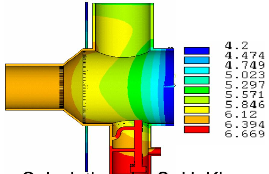
No significant difference in end groups' temperature profile in running at 4.2 K vs. 2.1 K
