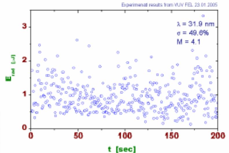
Multibunch SASE signal ( $\mu$ J) recorded with MCP Detector
