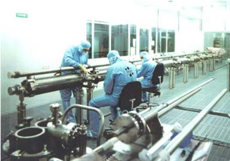
The assembly of an 8 cavity string has been continuously improved
