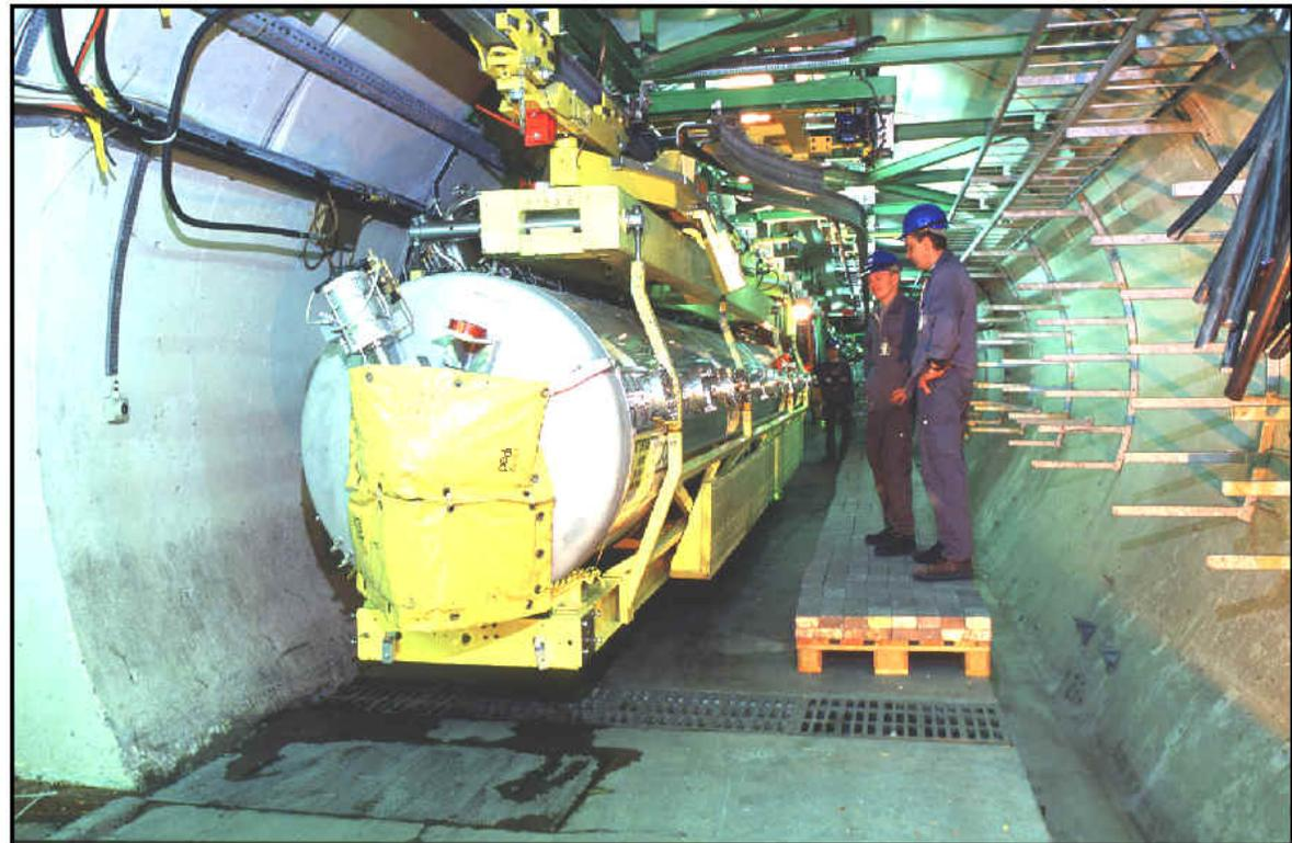
**Four cavities inside one vacuum vessel**
