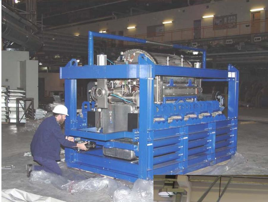
Special transport frame for shock absorption
