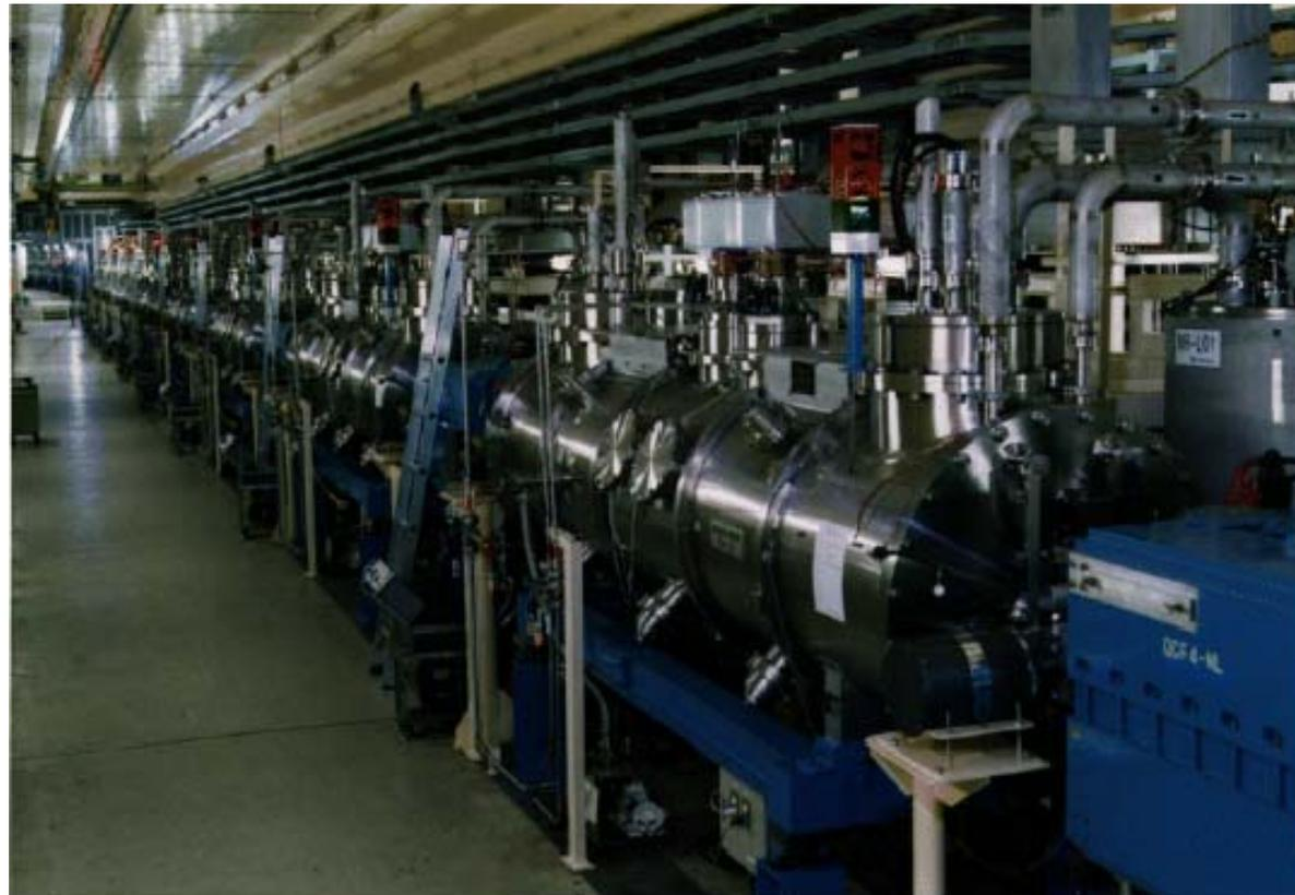
**Two cavities inside one vacuum vessel**
