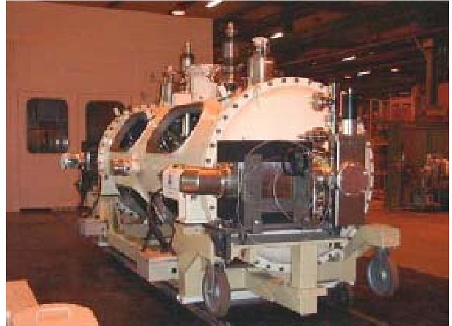
**Refurbished cryomodule prior horizontal test**
