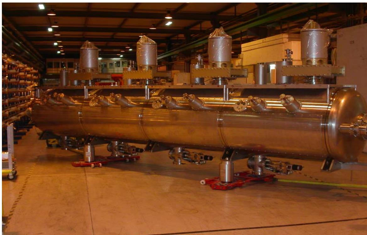
**Four single cell cavities (400 MHz) in one vacuum vessel**
