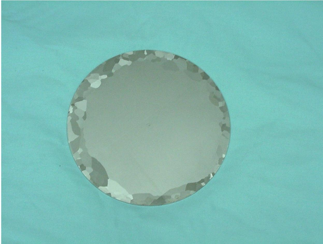
RMS Surface Roughness 27 nm per A. WU/JLAB on a 0.2 X 0.2 mm area
