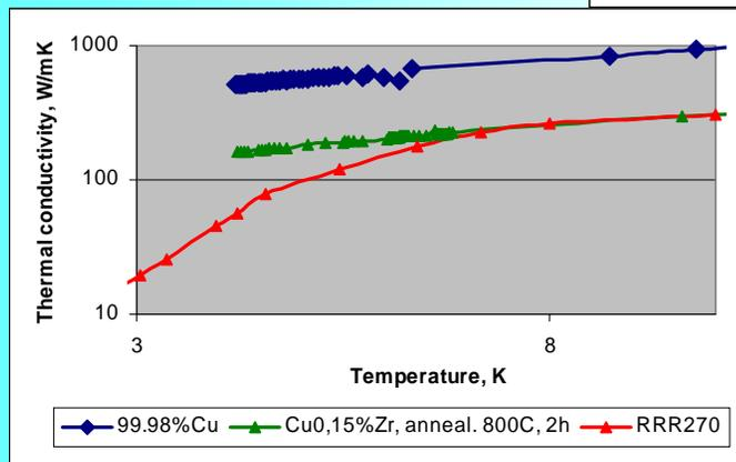
Thermal conductivity can be recovered by aging at ca.  $400^\circ\text{C}$ /one hour. Zr leaved the solid solution and creates precipitates  $\text{Cu}_5\text{Zr}$  finely distributed in Cu matrix
