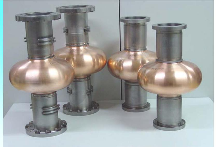
NbCu cavities hydroformed from explosively bonded tubes at DESY.
