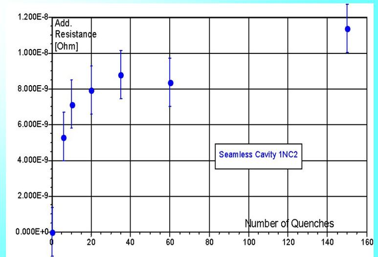
Additional surface resistance after quenches at ca 40 MV/m (P.Kneisel)
