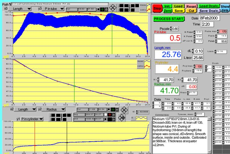
Front panel of the software for hydroforming - machine
