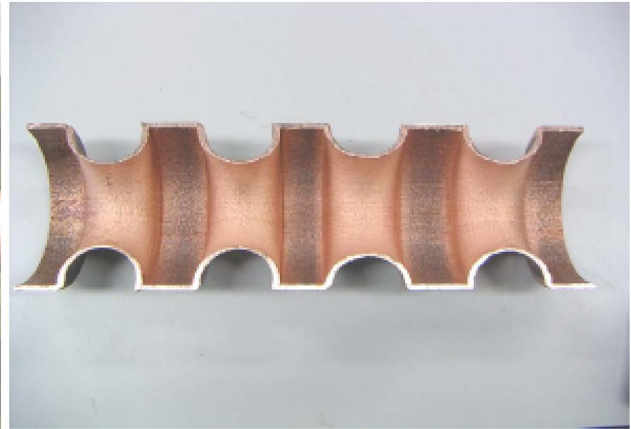
Necking 100phai, 3mm thick copper tube to 50phai
