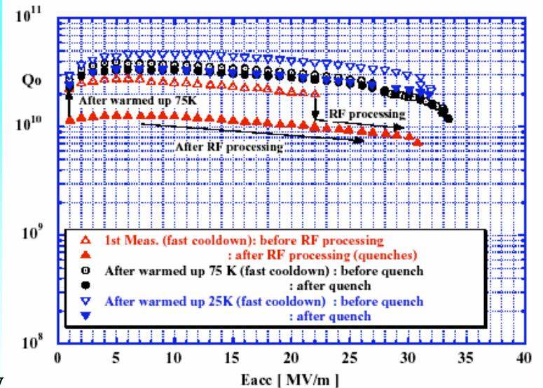
Q degradation in a seamless single cell cavity from NbCu explosively bonded tube (K.Saito)
