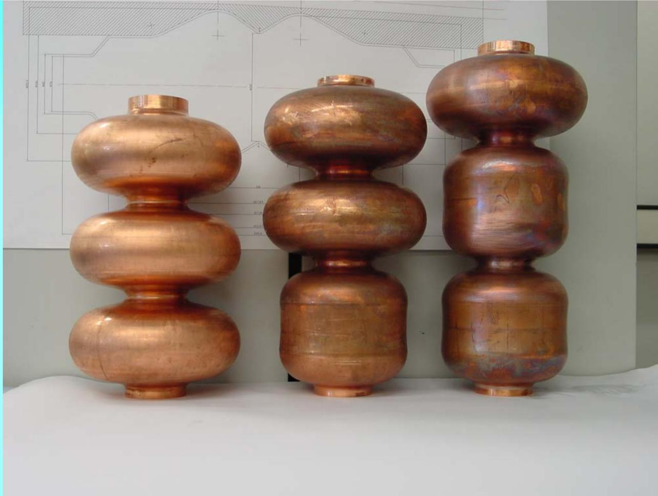
Hydroforming of cells can be done or as three cells simultaneously or cell by cell
