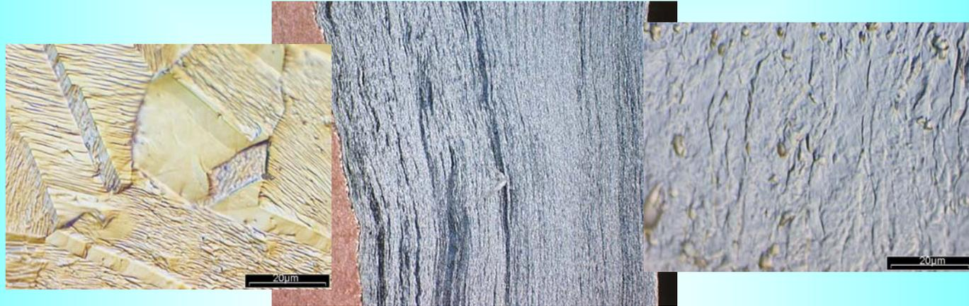
Microstructure of Cu and Nb after annealing at 560°C for 2 hours. Nb is not recrystallised (hard).
