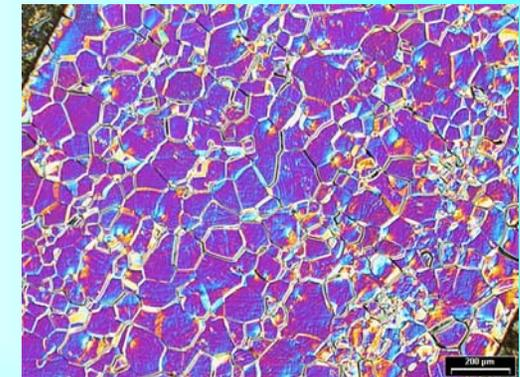
Appropriate microstructure and rather high strain before onset of necking. Tubes of 1,4 m long and ID ca. 200 mm for spinning have been build by V. Palmieri
