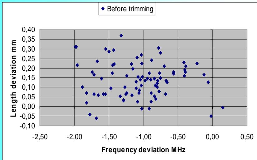
Example of dumb bells frequency for standard cavity fabrication
