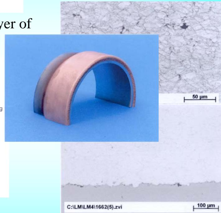
Microstructure of CGDS Cu coating on Nb, small porosity ca. 1%, small oxidation. electr. conduct. ca.80% of bulk Cu (top: spraying by Nitrogen, bottom- by Helium)
