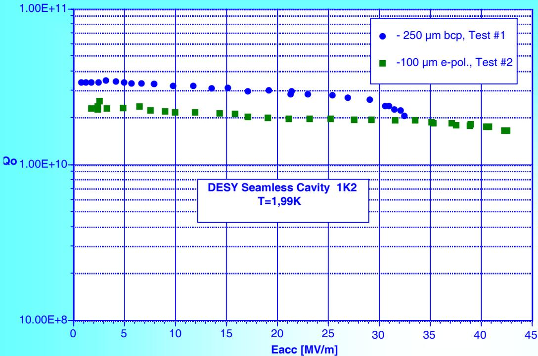
The best  $Q(E_{acc})$  result of by hydroforming produced single cell cavity
