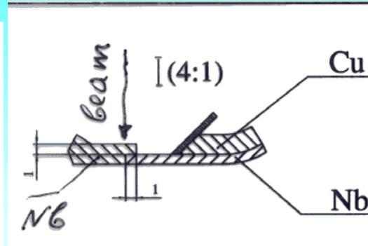
Cu layer on Nb tube. Small purity degradation of Nb during spraying: from RRR=300 to RRR=250
