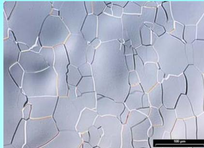
Microstructure of  $\text{Cu}_{0.15\%}\text{Zr}$  and Nb after annealing at  $800^\circ\text{C}$  for 2 hours.
