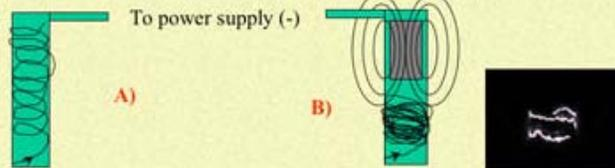
**A)** : The arc is started at the positive side of the cathode and stopped on a floating potential electrode mounted at the opposite side of the cathode itself. Alternatively the current flow can be inverted as the spot reaches the opposite cathode end.
