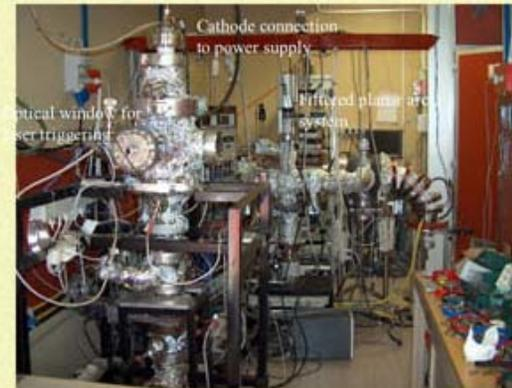
Laboratory in Rome: Cylindrical arc system and planar filtered arc
