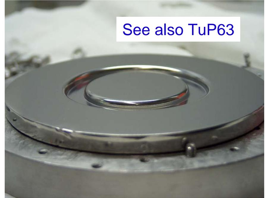
Cu samples with Nb ARC-coating. Used as a baseplate of 6 GHz cavity operating in the TE<sub>011</sub> mode. At low field, the surface resistance is in the range 3÷6  $\mu\text{Ohm}$ , as compared to the BCS  $R_s$  of 0.22  $\mu\text{Ohm}$  at 2.2 K and small mean free path. The Q remained constant up to a field of 300 Oe.
