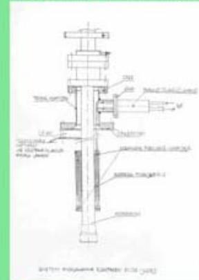
The filter, shown below, works as follows: a current driven through the copper tubing water cooled structure generating a magnetic field that
