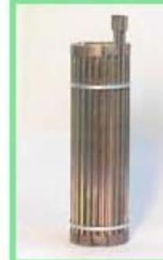
guides plasma electrons (and ions) through the small gaps between pipes. There being no direct line of sight from cathode to anode, heavy particles can instead not get through.
