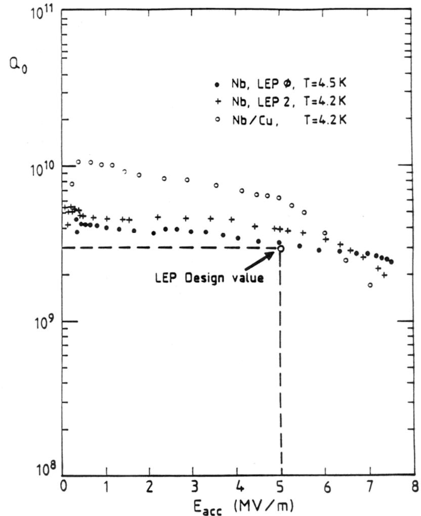
Fig. 2 Dependence of  $Q$  values on  $E_{acc}$ . Final values for 4-cell cavities LEP 0 and LEP 2 with  $H_{ext} \leq 160$  mG and for a 350 MHz 4-cell Cu-cavity with a magnetron sputtered Nb-layer.
