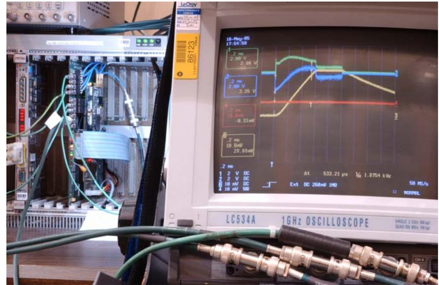
Using DESY's SimCon Series for LLRF control.
