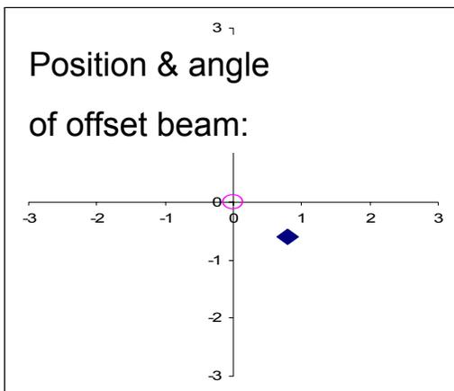
i.e. The 17<sup>th</sup> bunch, entering 0.5 mm away from the center loses  $\sim 200$ keV and is kicked 32  $\mu$ rad
