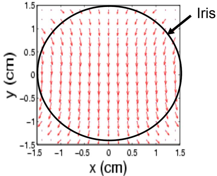
Uniformity map of the the integrated transverse kick along the the 13 cell cavity
