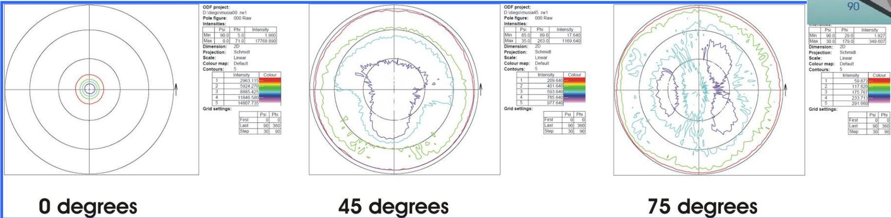
By cathodic arc, the substrate is biased; so ions always reach the substrate perpendicularly: **NO TEXTURE vs target-substrate angle**
