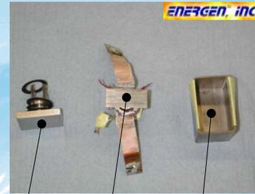
Ferrite necessary to close magnetic circuit
