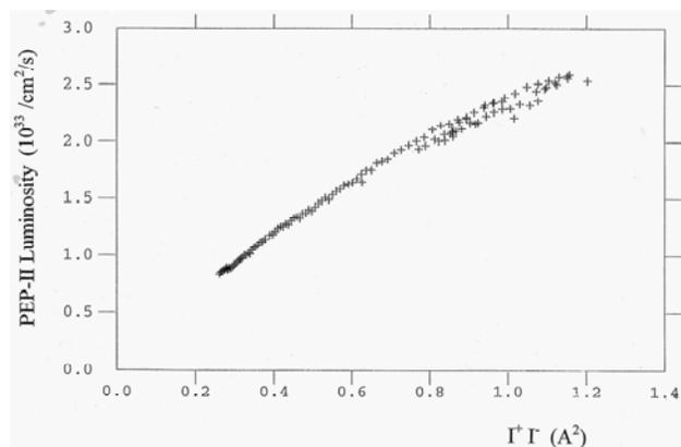
Figure 4. PEP-II luminosity versus the product of the beam currents. Note that the luminosity deviates from an ideal square law due to the enlargement of the beam sizes.
