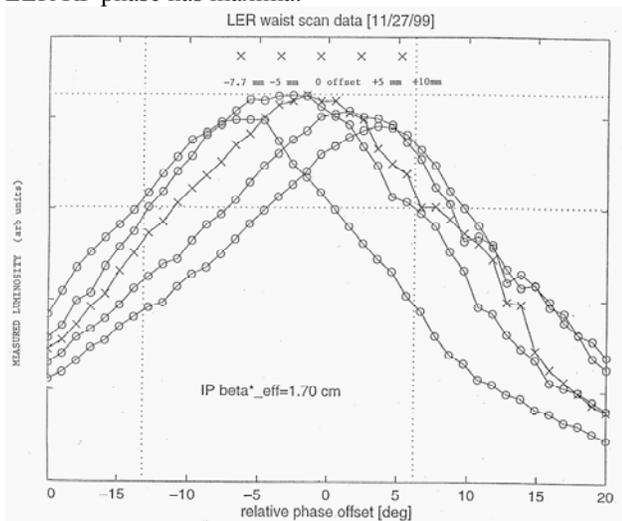
Figure 3. Variations in luminosity with HER RF phase as a function of location of the LER vertical beta waist.
