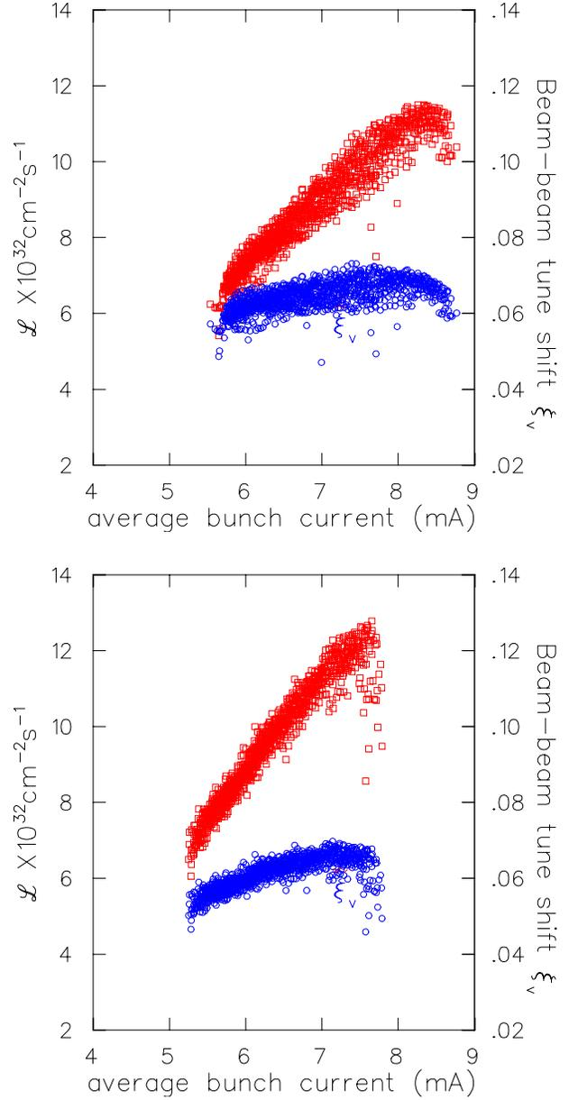
Figure 3: Beam-beam tune shift,  $\xi_v$  (blue circles), and luminosity (red squares) versus bunch current with nine 4-bunch trains/beam (top) and nine 5-bunch trains/beam (bottom).
