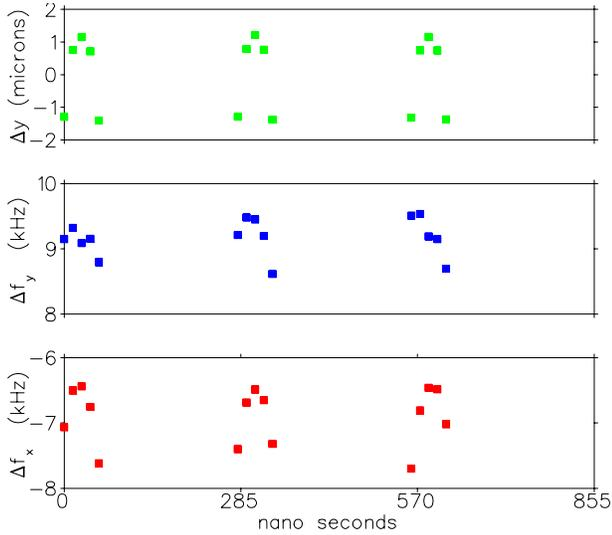
Figure 2: Calculated tune shifts in one beam due to the LRBBI with the opposing beam are shown in the bottom two plots. There are 9, 5-bunch trains with 7.5 mA/bunch in each beam and 14ns bunch spacing. The revolution frequency is  $f_{rev} = 390.1\text{kHz}$ . The difference in the vertical orbits at the IP for the two beams is shown in the top plot.
