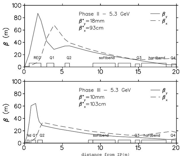
Figure 4: Betatron functions near the IP for CESR without (PHASE II) and with (PHASE III) the superconducting focusing magnets in the interaction region. For reference, the parasitic crossing nearest the IP occurs at 2.1 m.
