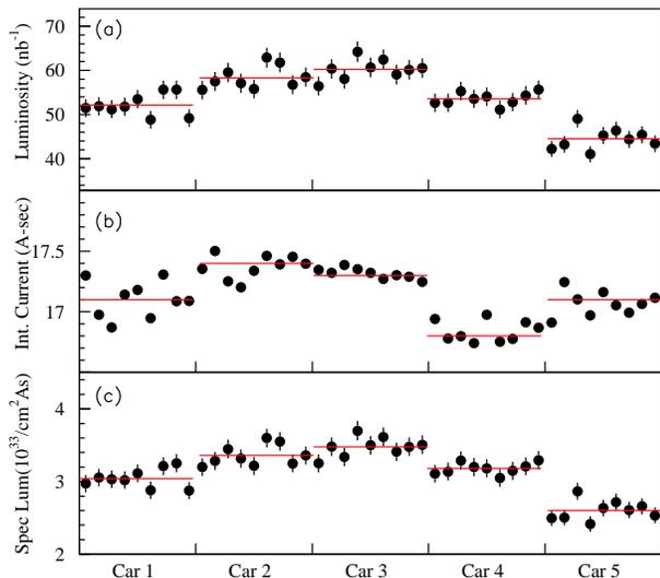
Figure 7: The (a) integrated luminosity, (b) integrated current, and (c) run-averaged specific luminosity of an HEP run with 9 trains of 5 bunches. The points represent the performance for individual cars while the lines indicate the average over all trains for each car.
