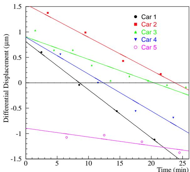
Figure 5: The vertical differential displacement for head-on collisions as a function of time as determined by maximizing the BBILM signal. The value for each car is averaged over all trains. The lines are linear fits to the data. The zero of the vertical axis is arbitrary.
