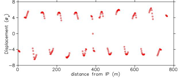
Figure 1: Horizontal displacement of the beam, in units of beam size, as a function of longitudinal coordinate in CESR. The displacement changes sign for the other species. At the center point in the plot, which is the crossing diametrically opposite the IP, the beams are separated vertically.
