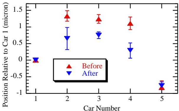
Figure 6: Positron - electron differential positions obtained with the CESR feedback system. The positions are averaged over all trains and are plotted relative to the average differential position obtained for car 1. The two sets of data were taken before and after adjusting the vertical positioning of all bunches using the feedback system's kicker.
