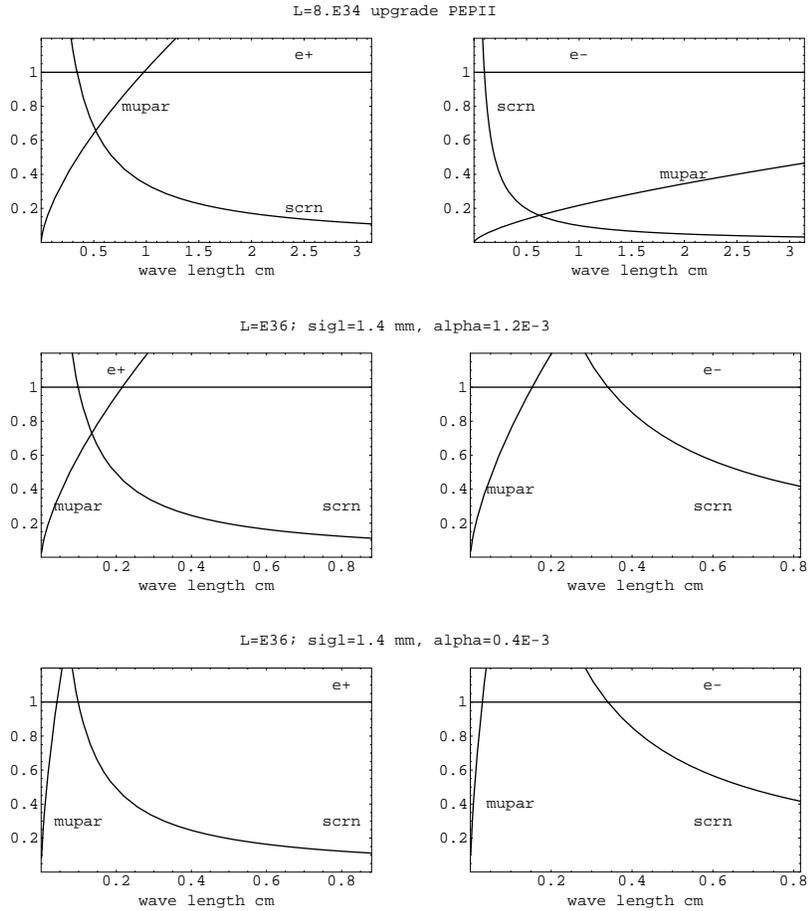
Figure 10: Parameters  $S$  and  $\mu_p$  for high-luminosity upgrades. In the last case, the CSR instability is possible.
