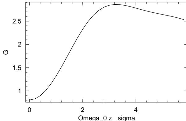
Figure 8: Variation of the tune shift along a long bunch.  $p = 0.2$ ,  $\Sigma_{x,y}/\sigma_{x,y} = 5$ .
