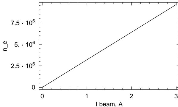
Figure 1: *The estimate of the average electron cloud density per  $\text{cm}^3$  as function of beam current.*
