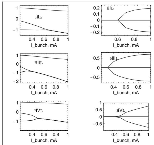
Figure 9: *The threshold of the head-tail instability for upgrades of the PEP-II. In the left column: the tune shift  $\Omega/\omega_s$ , vs. bunch current. In the right column: the dimensionless growth rate  $1/(\omega_s\tau) = \text{Im}(\Omega/\omega_s)$ . The rows are for the II, III, and IV upgrade parameters, see Table 3, respectively. The density of the cloud is scaled proportional to the beam current. Parameters of the wake are explained in the text.*
