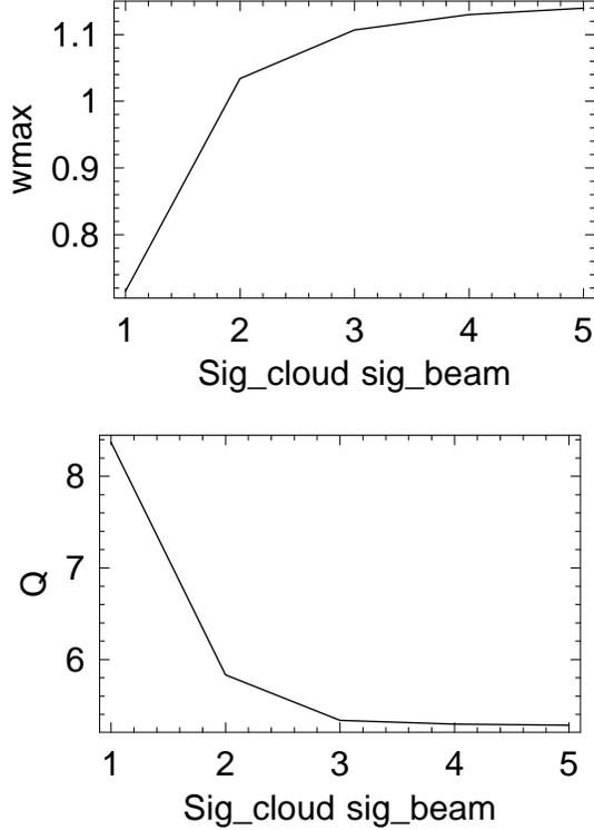
Figure 5: *Dependence of  $W_{eff}(\zeta, 0)$  on  $\Sigma_{x,y}/\sigma_{x,y}$  for fixed  $p = 0.2$ .*
