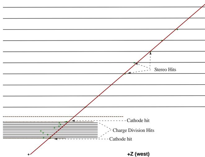
FIGURE 2.  $r - z$  View. Charge division wire hits are ignored. Tracking program looks for stereo or cathode hits to make a track. The DR axial wires and the PT detector have been removed for clarity
