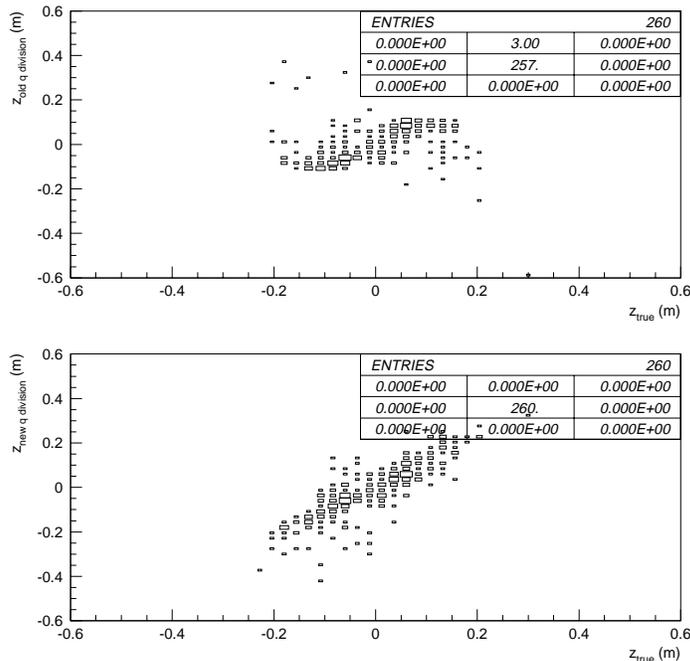
FIGURE 9. At top is the true  $z$  vs. charge division  $z$  of the cubic fit. At the bottom is the same for the linearized cubic. We see a diagonal at the bottom. Here, the charge division  $z$  is nearly the same as the true  $z$ . At the top, however, the cubic fit changes the course of the charge division  $z$  position; thus, the true  $z$  and charge division  $z$  do not match.
