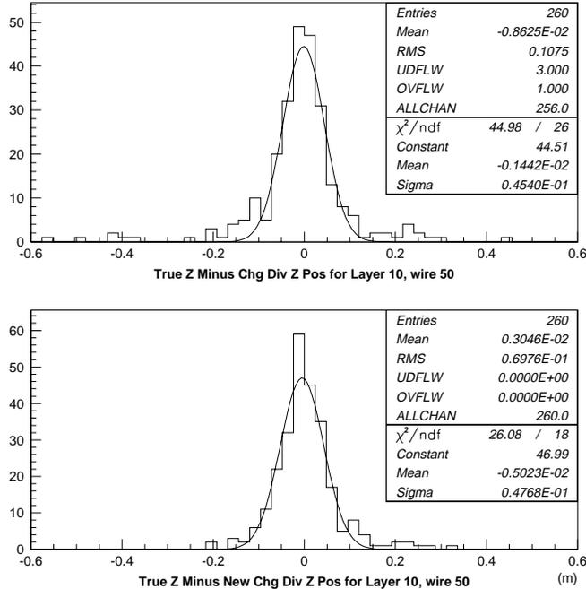
FIGURE 8. This plot shows the difference of the true  $z$  position and the measured charge division  $z$  position. The top shows the cubic fit. The bottom shows the linearized cubic which scales down the tails shown in the top plot and shows a better fit to the Gaussian.
