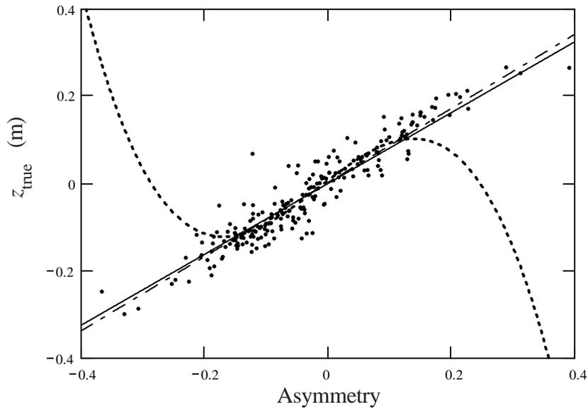
FIGURE 6. This plots shows the comparison of the cubic fit (dotted line), a linear fit (dashed line), and a linearized cubic fit (solid line). The points are the all the hits on the wire instead of just the hits in the calibrated region. The linearized cubic is very close to the linear fit.
