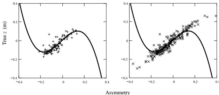
FIGURE 1. Two plots from CLEO II  $\mu$ -pair data showing true  $z$  vs. asymmetry for charge division hits on one wire. The points are the hits and the line is the cubic calibration fit. On the left is only hits in the calibration region. On the right are all the hits on the wire.
