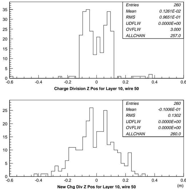
FIGURE 7. The top plot shows the  $z$  position using the cubic fit. There is a sharp cutoff on both sides. The cutoff on the sides is due to the turn of the cubic fit. The bottom shows the  $z$  position using the linearized cubic of Eq. (3) removing the cutoffs.
