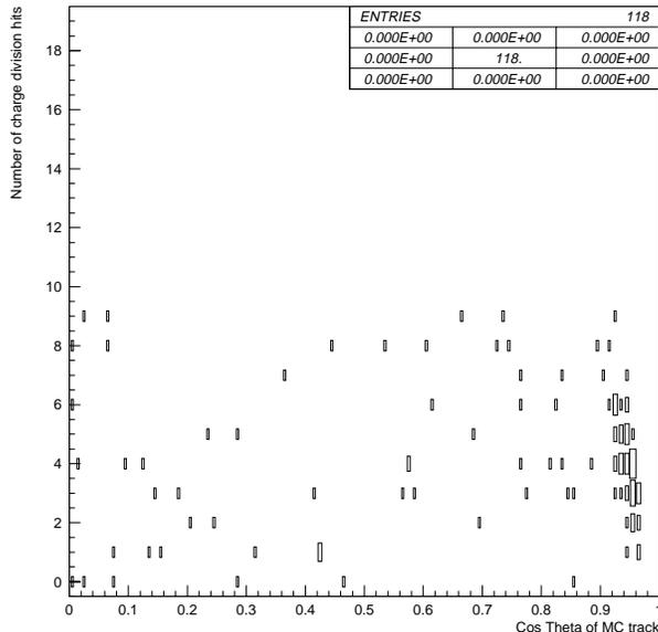
FIGURE 3. From CLEO II  $\mu$ -pair data shows the number of charge division hits vs.  $|\cos(\theta)|$ . After doing a distance of closest approach (dca) cut (less than 1 cm) and requiring that the tracks are not curler or ghost tracks, we found the forward tracks the tracking program indicated had no  $z$  fit did have charge division hits with  $z$  information.
