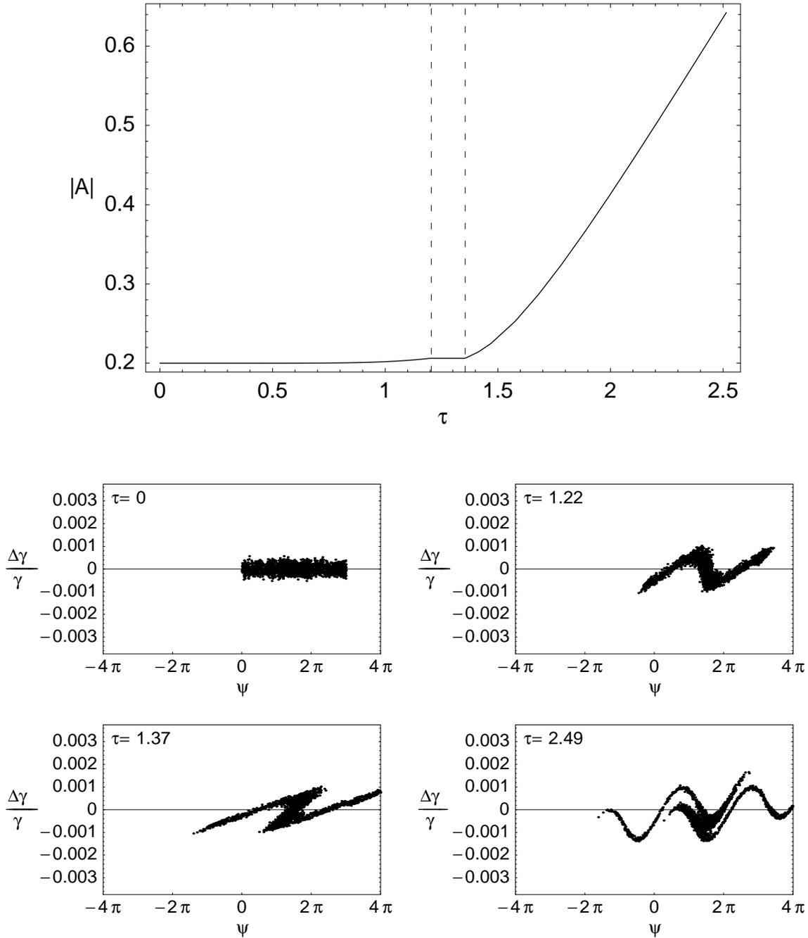
**FIGURE 2.** Typical FEL oscillator single-pass simulation conducted with 2,000 electrons. The radiation field amplitude  $|A|$  is given a large initial value of 0.2, as might be the case after field buildup over a number of passes, to demonstrate the effect of the dispersive magnet more clearly. The dashed lines on the field plot indicate the start and end of the dispersive magnet. The lower figures illustrate the evolution of the electron longitudinal phase space.
