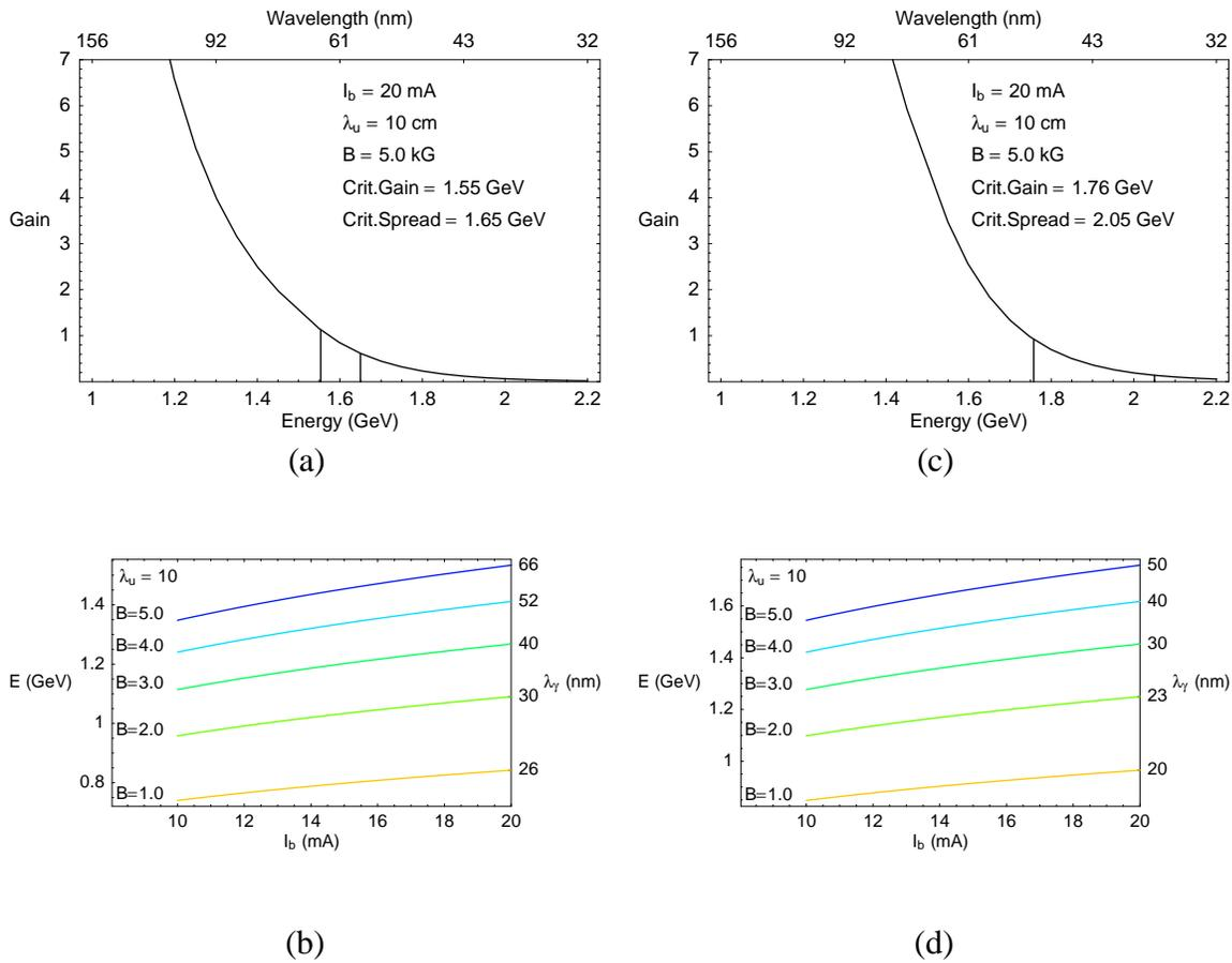
**FIGURE 3.** Parameter space for storage ring FEL oscillators. Figs. 3a & 3b show the parameter space for a single 15m undulator, while Figs. 3c & 3d describe an OK with a pair of 7.5m undulators and a 1m dispersive magnet. The upper plots illustrate the critical gain and spread criteria for a particular system, and the lower plots show various critical energy contours for different undulator magnetic field settings.  $\lambda_u$  is presented in cm, and  $B$  in kG.
