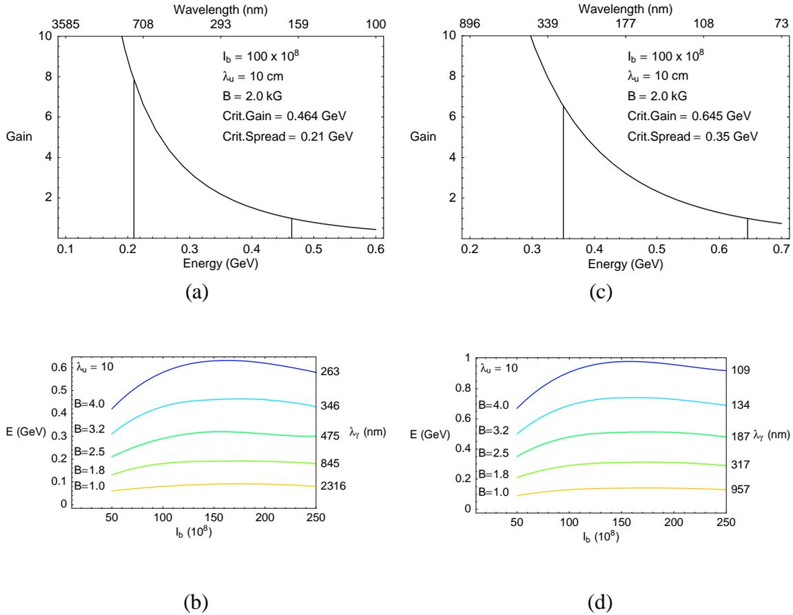
**FIGURE 4.** Parameter space for linac FEL oscillators. Figs. 4a & 4b show the parameter space for a single 15m undulator, while Figs. 4c & 4d describe an OK with a pair of 7.5m undulators and a 1m dispersive magnet. The upper plots illustrate the critical gain and spread criteria for a particular system, and the lower plots show various critical energy contours for different undulator magnetic field settings.  $\lambda_u$  is presented in cm, and  $B$  in kG.
