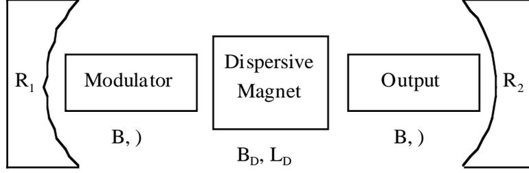
**FIGURE 1.** Schematic of a complete FEL oscillator. The electron beam enters at the modulator (undulator magnet) and exits after the output section.
