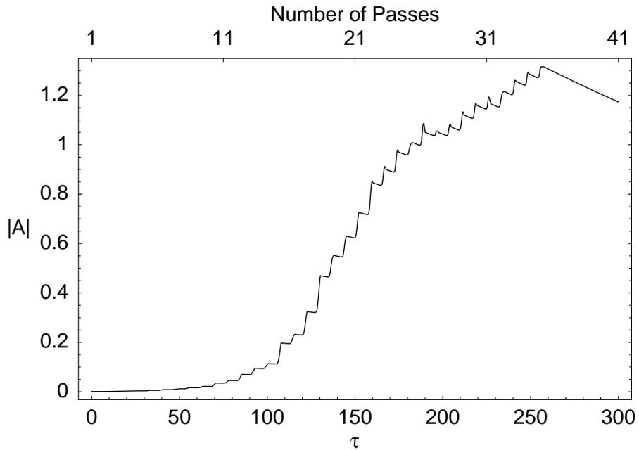
**FIGURE 6.** Radiation field amplitude for a 15m FEL in a 17m cavity. Mirror reflectances are  $R_1=0.98$ ,  $R_2=1.0$ . Simulation was conducted with:  $E = 320$  MeV,  $\lambda_u = 10$  cm,  $B = 2.5$  kG,  $I_b = 2.5 \times 10^{10}$  electrons. Radiation wavelength is 475 nm.
