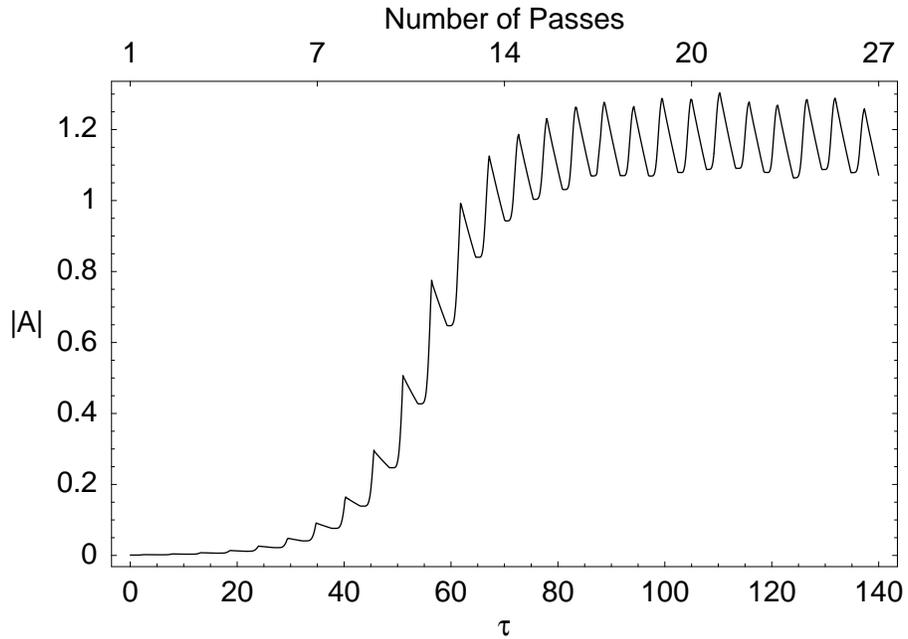
**FIGURE 5.** Radiation field amplitude for a 15m FEL in a 17m cavity. Mirror reflectances are  $R_1=R_2=0.85$ . Simulation was conducted with:  $E = 1.4$  GeV,  $\lambda_u = 10$  cm,  $B = 4.0$  kG,  $I_b = 20$  mA. Radiation wavelength is 52 nm.
